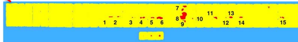
Acceptable defects/UT examination
